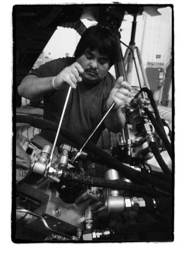
Richard Rocha is practicing some "artery surgery" on the hydraulic system powering one of the legs of the Motion Based Space Shuttle Simulator which needs to be replaced. The operation will last about 5 hours and require the efforts and expertise of 3"surgeons."
