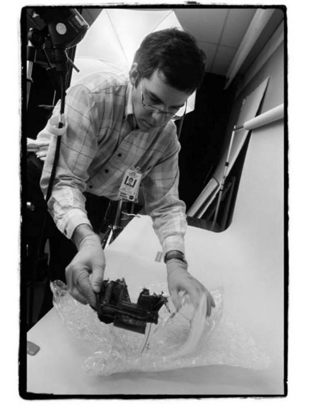
A terribly tormented debris of what used to be one of the cameras of *Columbia's* crew made its way from East Texas to JSC photo lab for documentation and identification.
